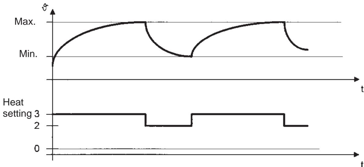
The maximum heat settings and minimum temperature values (NTC R2, NTC R3) permitted for a programme section have been defined in the drying programme. Both temperatures are monitored in parallel, the reset temperature having higher priority.
