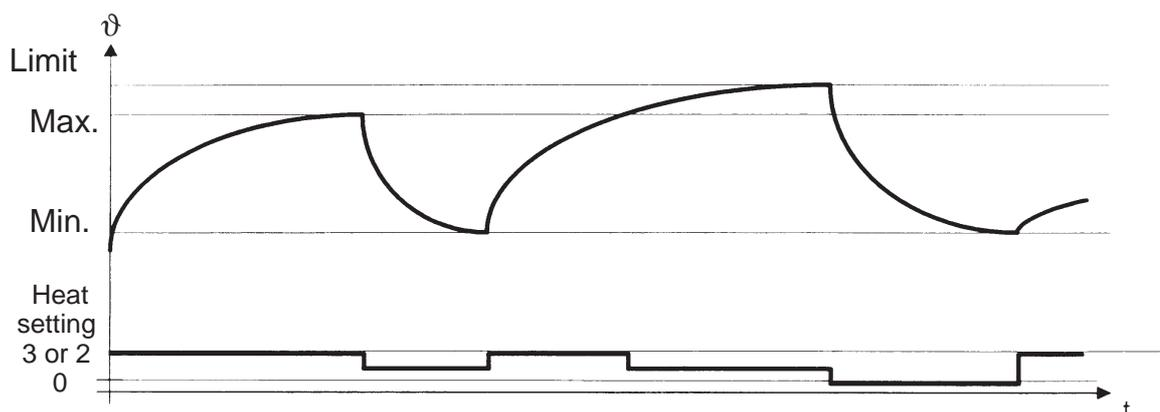
If the temperature limit is exceeded, all heaters are switched off. The heater is not switched on again until the temperature has dropped to  $\vartheta$  min. If the temperature does not drop below the temperature limit within 10x30 sec., the drying process is terminated and an "Overheating" error message (extra dry LED) is output.
